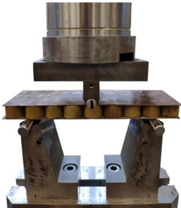
Fig. 6. Characterisation of the sandwich panel via three-point bending test.
