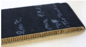
Hemp/Polyamide skins with Paper Honeycomb Core
