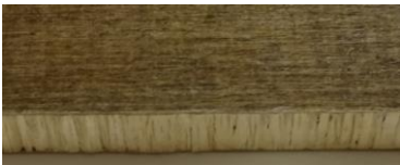
Flax/Epoxy skins with Lightened Balsa Honeycomb Core
