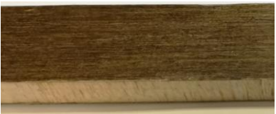
Flax/Epoxy skins with Balsa Core
