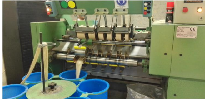
(b) Drawn sliver at the output of the second stage
