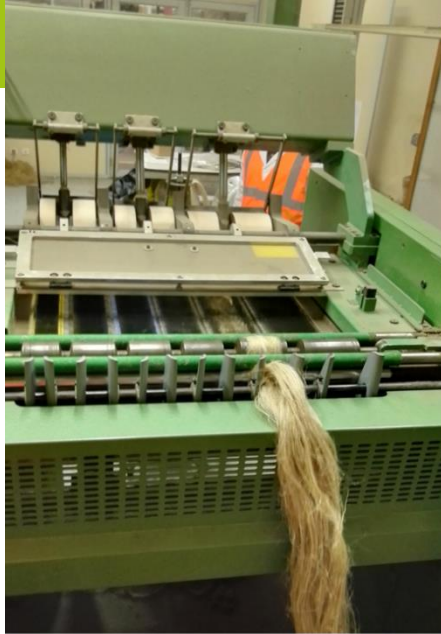
(a) Sliver input into the gill system
