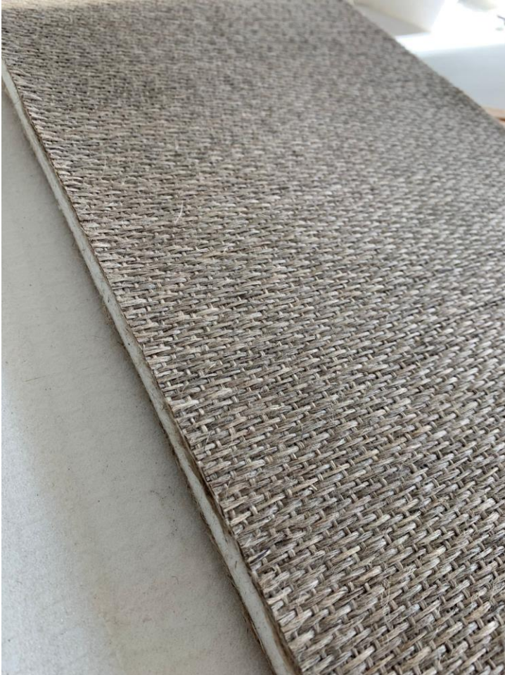
PET & SSUCHY FLAX DRY PACK ON HOT PLATE
