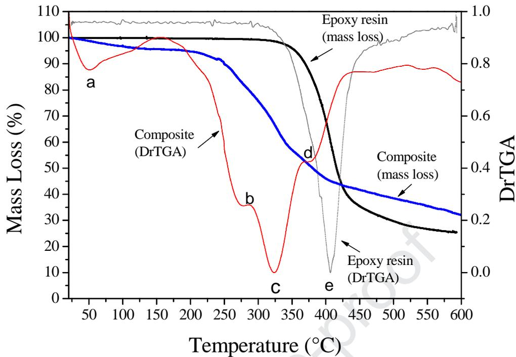
Figure 5. Thermogravimetric analysis for epoxy polymer and flax composite.
