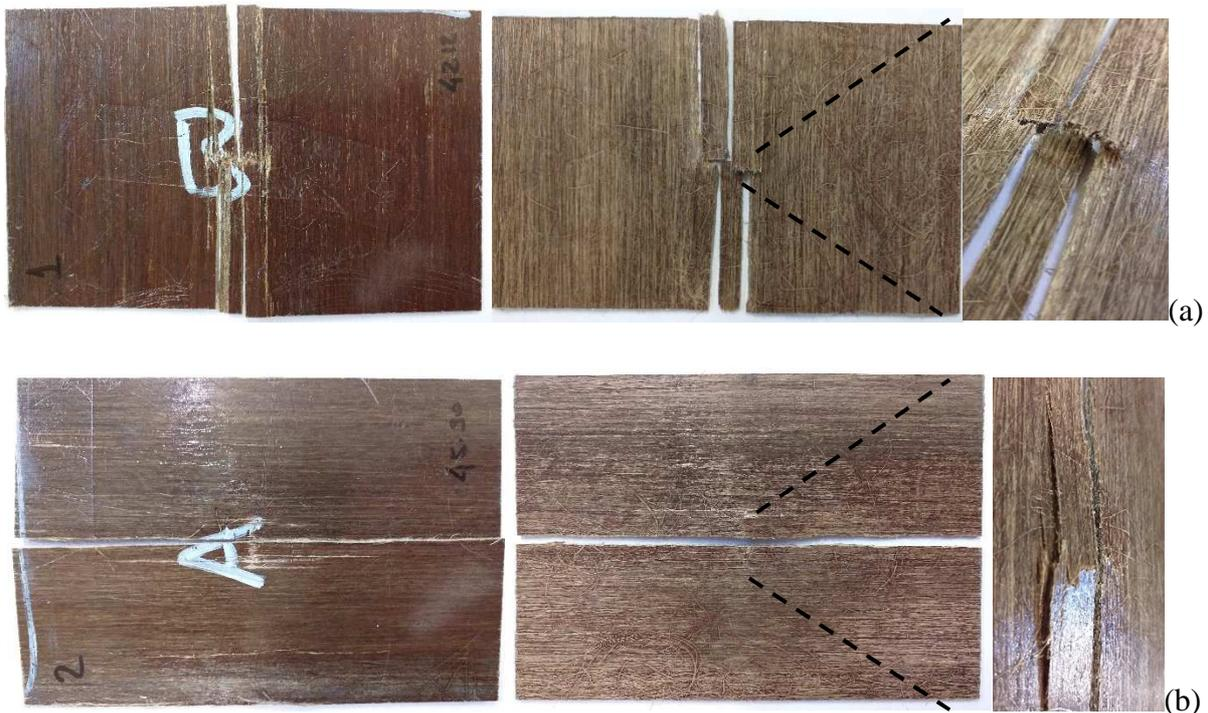
Figure 15. Impact specimens after testing: (a) transverse and (b) longitudinal fibre directions.
