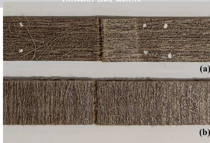
Figure 7. Tensile fractures of samples tested in longitudinal (a) and transverse (b) directions.
