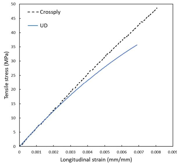
Figure 12. Mechanical behaviour of UD and crossply flax composites under shear load via tensile testing.
