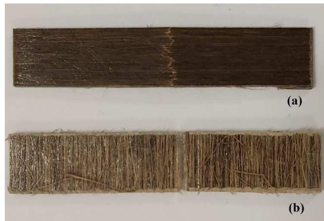
Figure 11. Bending fractures of samples tested in longitudinal (a) and transverse (b) directions.
