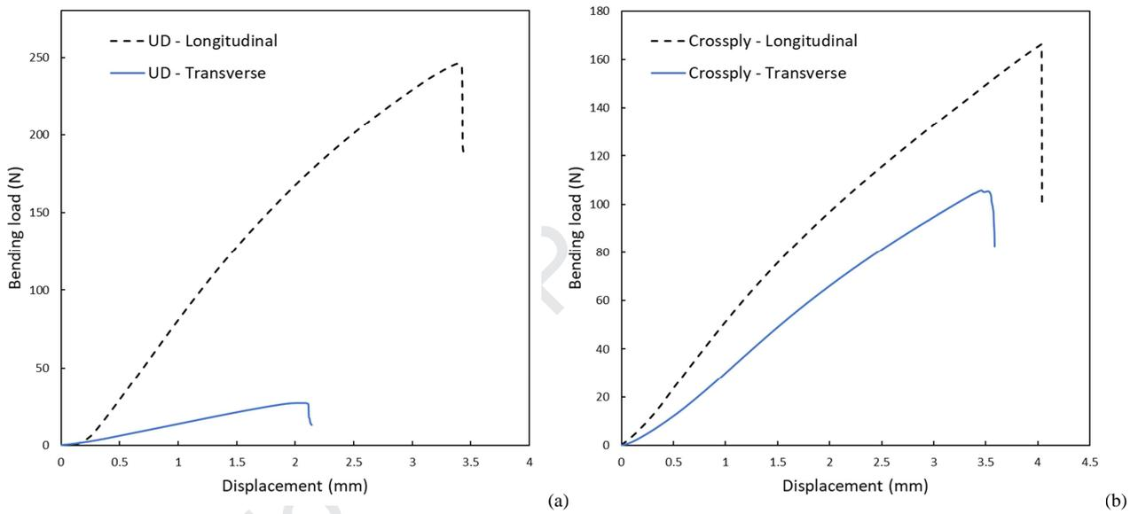
Figure 10. Typical bending behaviour of UD (a) and crossply (b) flax composites.
