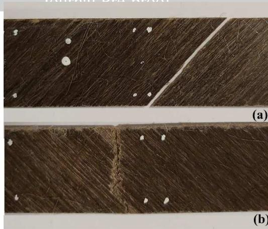
Figure 13. Shear fractures of UD (a) and crossply (b) samples.
