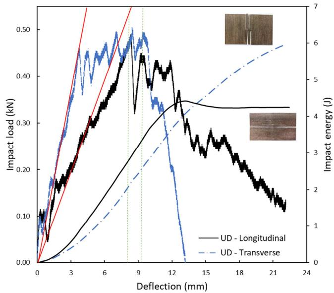
Figure 14. Impact responses for typical UD samples tested in the longitudinal and transverse fibre directions.
