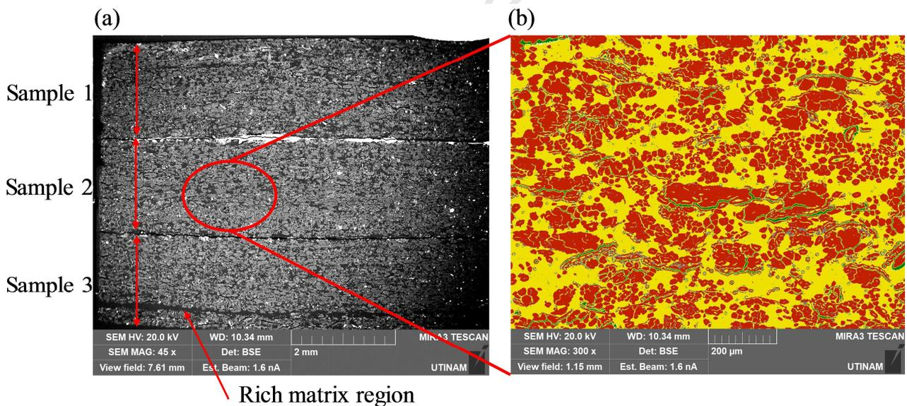
Figure 3. SEM image of 3 unidirectional [0]<sub>12</sub> specimens in the cross-section (a) and processed image of a specific area (red = fibres, yellow = matrix, and green = porosity) (b).
